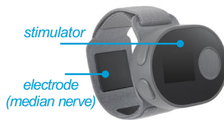
Figure 1 Wrist-worn TAPS device, including stimulator, two working electrodes (median and radial nerves), and one ground electrode.
